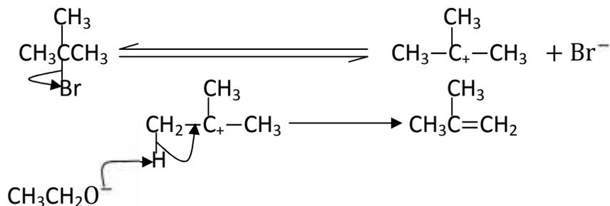
(b) Primary alkyl halide react with hot alcoholic solution of potassium or sodium hydroxide to form an alkene. The reaction is bimolecular elimination ( $E_2$  reaction)
